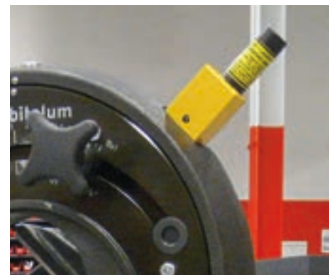
Integrated laser Indicates cut-off point
