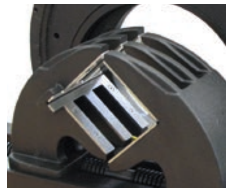
Deformation free stainless contact clamping jaws
