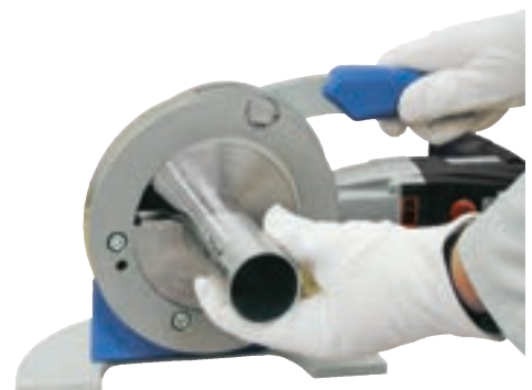
RPG 4.5 securely clamps to tube
