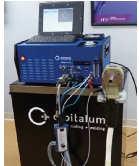
Arc Machines (AMI) Weld Head Connected to Orbitalum OM 165CA Orbital Welding Power Supply
