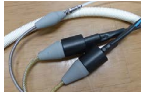
AMI Adapter Cable Connections feature protective sleeves
