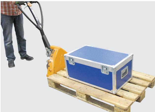
Transport in packaged condition on a pallet with suitable lifting equipment (e.g. lifting truck).
