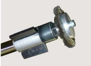
These brass brush attachments prevent chips and other foreign bodies from inadvertently falling into the inside of the pipes, making them particularly useful for vertical work on containers.
