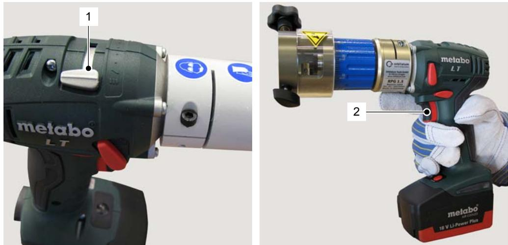
**Increasing speed** ▶ Press the speed regulator (2) further down.
