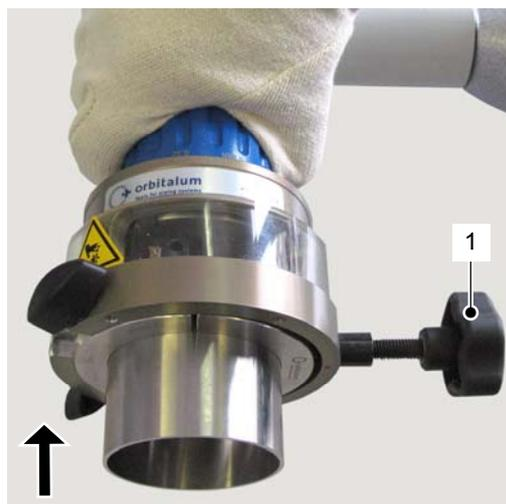
*Clamp tube with RPG Electric:
